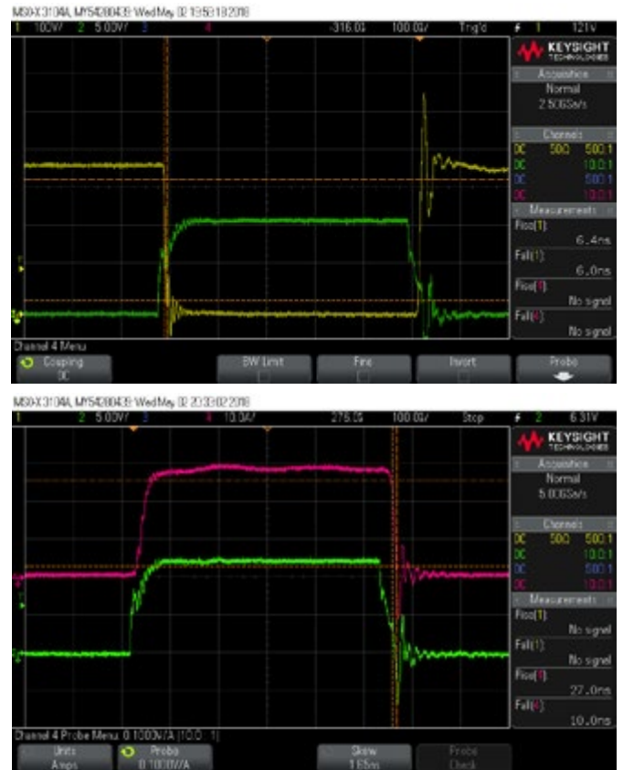
Figure 3: Experimental measurements of the GaN (VisIC V22N65A). (a) Driver signal (Green) and VDS (yellow) at current ‘turn off’. (b) Driver signal (Green) and ID (red) of GaN at current ‘turn on’.
