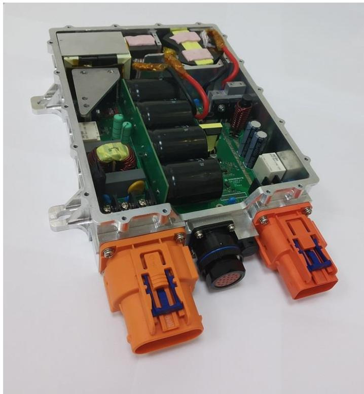
The 6.7kW OBC using VisIC GaN power devices targets plug-in hybrid vehicles/electric vehicles (PHEV/EV) applications. With a universal 110-220V/16-32A AC input and 200-430V DC output for charging the automotive battery by controlling voltage and current flow to the battery. The charger is designed to provide the interfaces to charging standards on the input power side and thus adapts to charging infrastructure.
